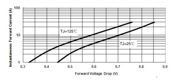
Fig.3-Typical Instantaneous Forward Voltage Characteristics
