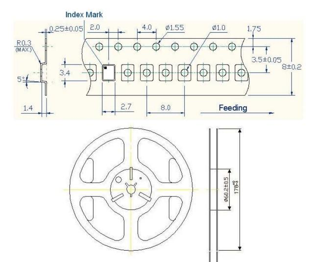
1. 230mm minimum leafer which consist of carrier and/or tape followed by a minimum of 160mm of empty carrier tape sealed with cover tape.
