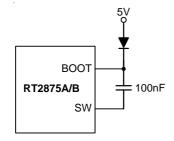
Figure 2. External Bootstrap Diode
