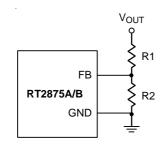
Figure 1. Output Voltage Setting
