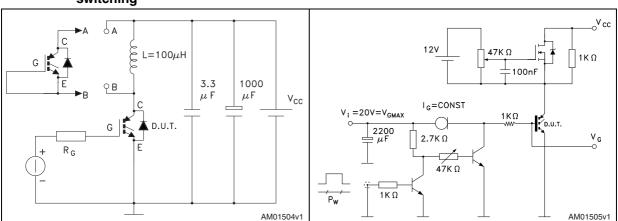
Figure 17. Test circuit for inductive load switching
