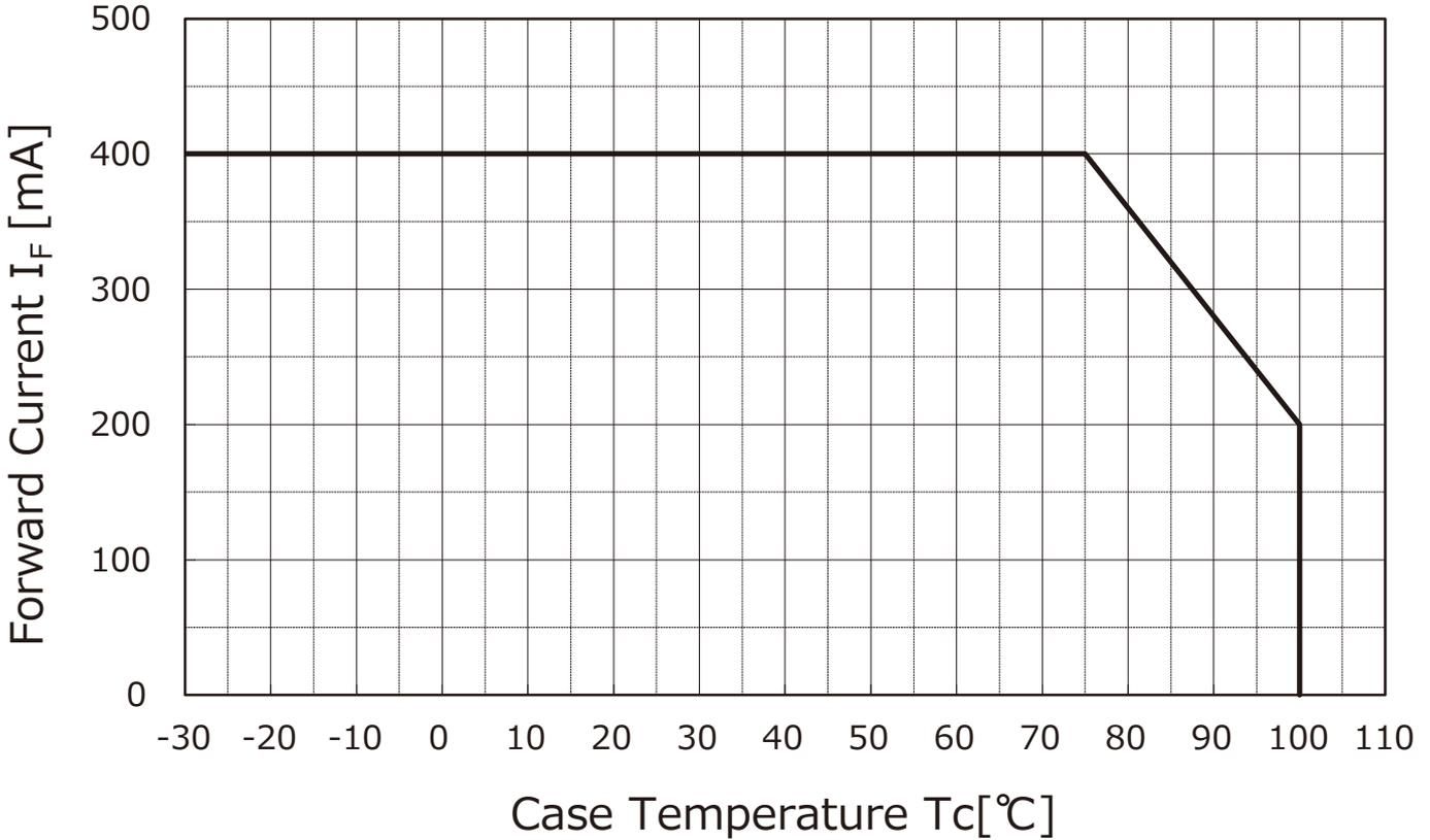
(Note) To keep the case temperature lower than the rating, enough heat-radiation performance needs to be secured by using an adequate heat sink (refer to section 7-③).
